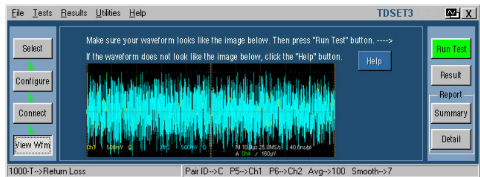
Figure 11-8: 1000BASE-T View Waveform for Return Loss
