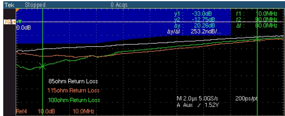
Figure 9-18: Waveform for 100BASE-TX Return Loss Transmitter
