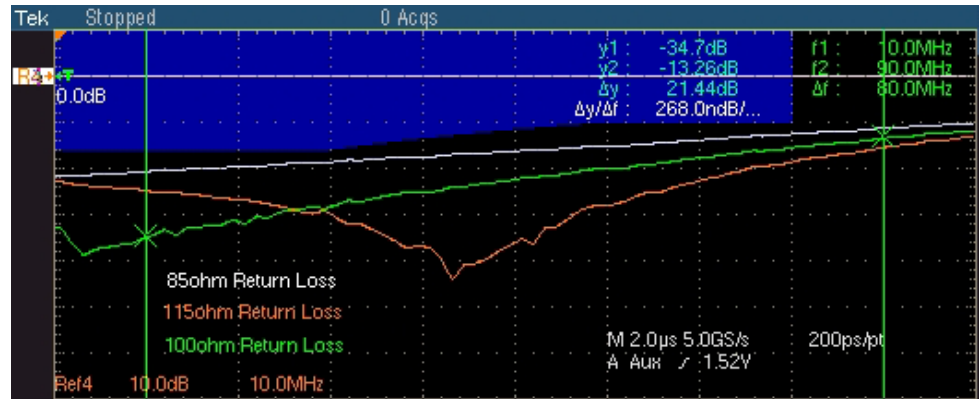
Figure 9-19: Waveform for 100BASE-TX Return Loss Receiver
